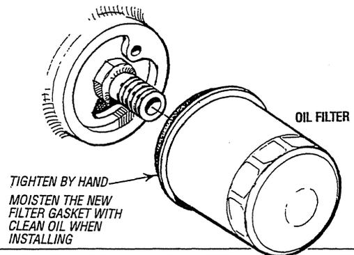
**WARNING:** Used engine oil contains harmful contaminants. Avoid prolonged skin contact. Clean skin and nails thoroughly using soap and water. Launder or discard clothing or rags containing used oil. Discard used oil properly.
