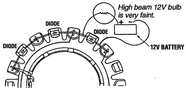
6. **Rotating Field Windings 7.0-8.0 ohm.** Readings taken between the two red & white wires connected to the (+) and (-) terminals of the exciter rotor as shown.
