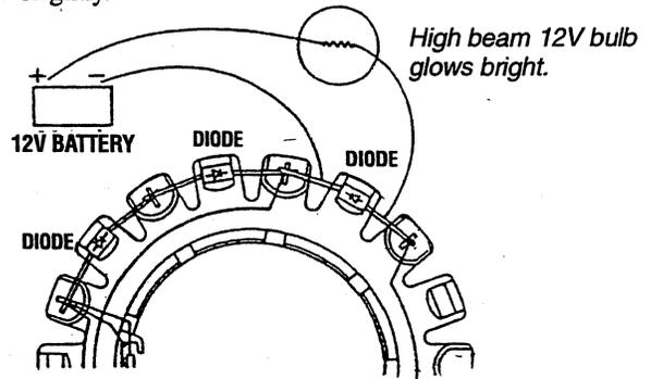
5. **Reverse the leads across the diode.** The diode should block voltage passing through it, and the headlight should not glow, or it may glow faintly.
