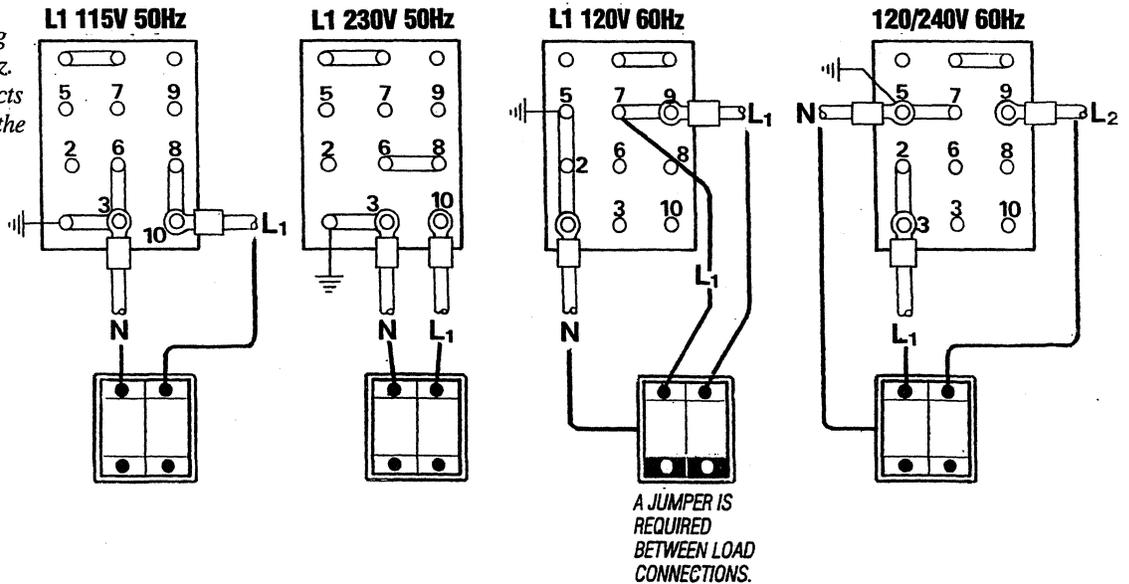
**NOTE:** For output leads from the AC terminal block use terminal ends for 1/4" studs that accept multi-strand copper wire sized for the average rating from the hot lead connection
