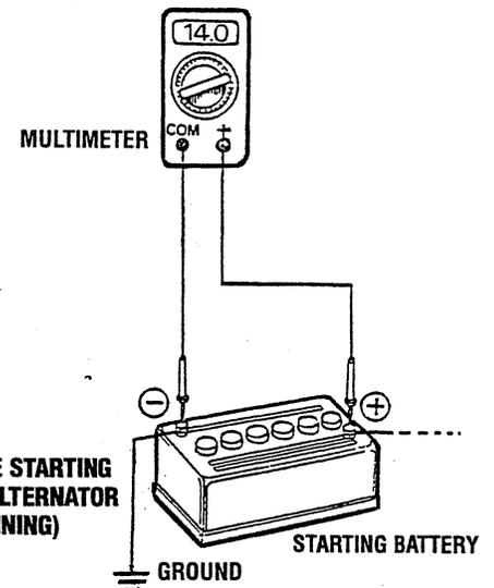
3. If the starting battery voltage remains around 12 volts after the engine is started and run for a few minutes, a problem exists with the alternator or the charging circuit.
