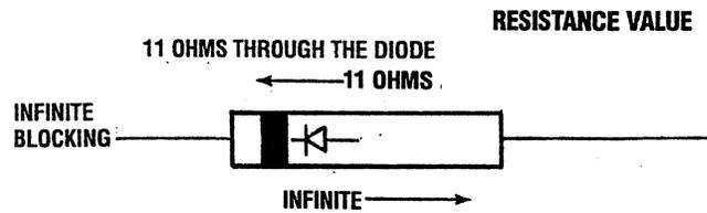
**NOTE:** Attempting to check diodes in place with an ohmmeter will give erroneous readings on the diodes due to the auxiliary winding's connections.
