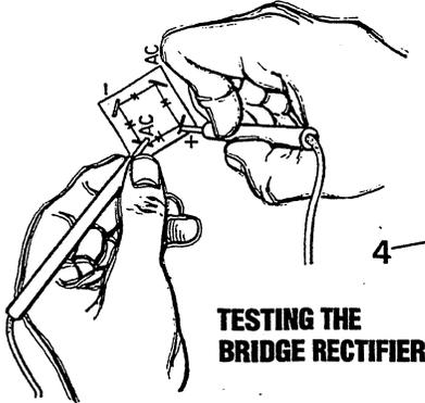
**TESTING THE BRIDGE RECTIFIER**
