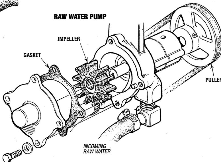
**CAUTION:** If any of the vanes have broken off the impeller, they must be located to prevent blockage in the cooling circuit. They often can be found in the heat exchanger
